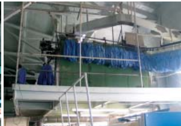
Scrubs and other apparel move on a conveyor after processing in the tunnel finisher.
